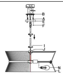
Step 4: Then use the round nut (F) to lock the canopy (E) onto the mounting plate (B), and insert the bulb (N) into the socket of the shade A (J)
