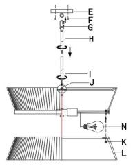
Step 2:Lock lampshade B (L) onto lampshade A (J) with nut (K), then rotate the long tube (I) and short tube (H) clockwise onto lampshade A (J), and then lock the C-ring (G) onto the short tube (H) and canopy (E).
