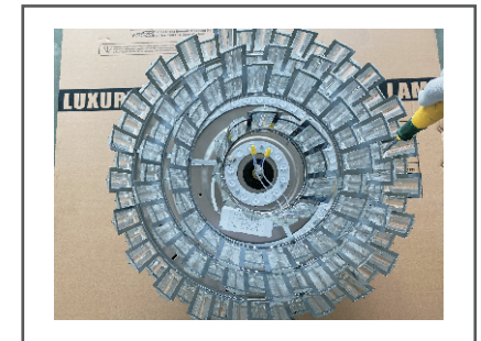
Step 9. Install and fix the lampshade on the chassis with screws.
