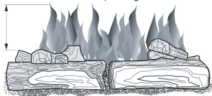
Figure 20 - Incorrect Burner Flame Pattern
