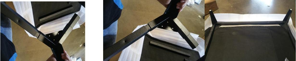
Step 3. Once everything is inserted use a screwdriver to tighten the screws on the sofa frame to hold the legs/frame in place.
