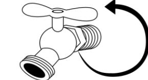
2) Wrap the tape around the threaded end of the spigot in a counterclockwise direction.
