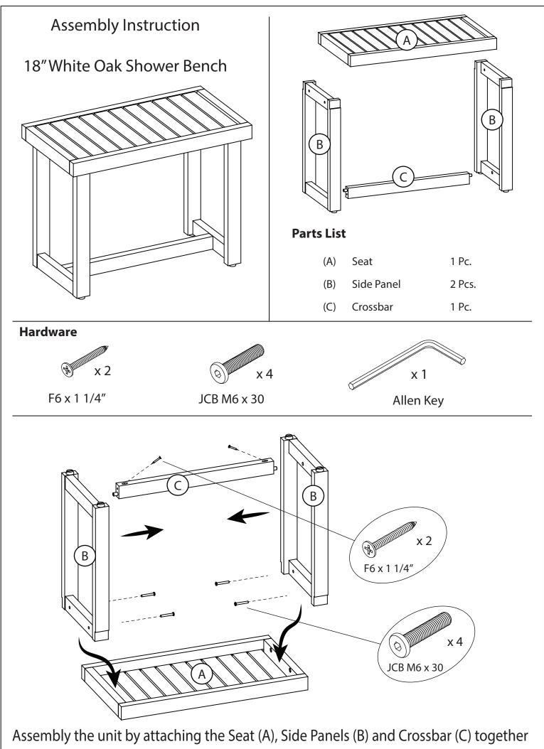
by using Screw JCB M6 x 30 and Screw F6 x 1 1/4" as shown in diagram.
