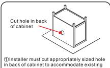
placement of hot & cold wall valves and drains,
