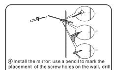
the holes and insert the plastic wall anchors.
