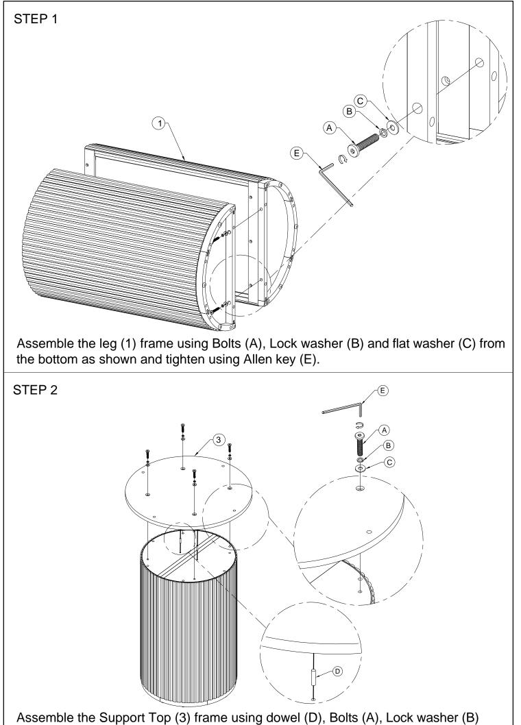
and flat washer (C) from the bottom as shown and tighten using Allen key (E).
