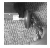
4) Tighten the bolt with a wrench.
