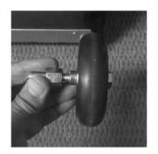
2) Insert bolt through wheel and attach nut. Make sure to thread nut onto the bolt on the side with raised part of the wheel housing.
