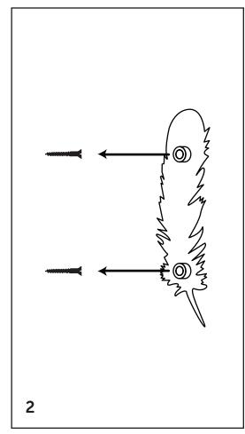
Place two screws into wall surface.
