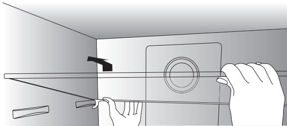
2. To reinstall a shelf, rest the shelf on both the front and rear supports. Push the shelf toward the rear of the refrigerator until the back of the shelf hooks around the rear shelf supports.
