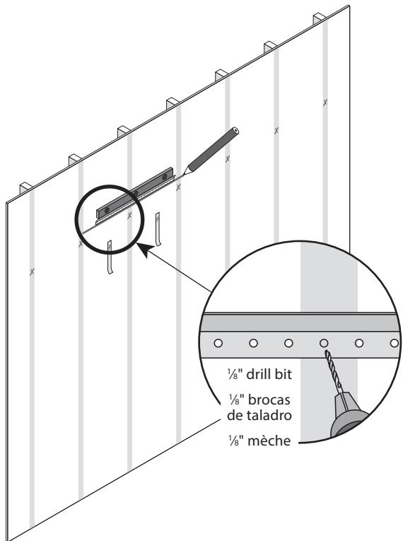
**6** **IMPORTANT.** If a vertical will be more than 3" from a stud, you'll need to use a toggle to support that panel. Mark toggle locations next to vertical panel locations. If panel will be less than 3" away, skip to Step 9.
