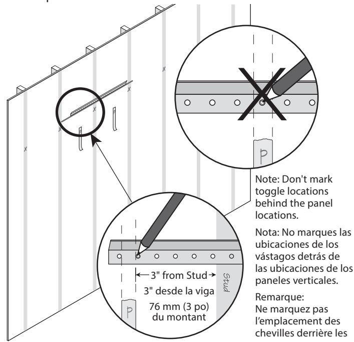
**7** Rotate rail out of position, then drill toggle holes. Use  $\frac{1}{2}$ " drill bit.
