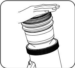
Step 3 Place your hand over the bean hopper lid, then gently press the air blower to expel any remaining coffee grounds from the grinder.
