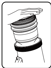
2. Press the air blower to expel any residual coffee grounds from the grinder.
