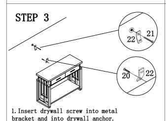
2. Insert flathead screw into second metal bracket and into back of item. along top edge.
