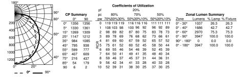
2BLT4 48L ADP LP835, 5121 delivered lumens, test no. LTL28918P41, tested in accordance to IESNA LM-79
