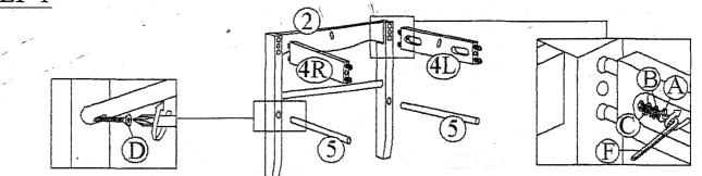
Use allen key (F) , JCBC screw 50MM (A) , spring washer (B) and flat washer (C) to assemble left and right side apron (#4L & 4R) to chair front leg (#2) .
