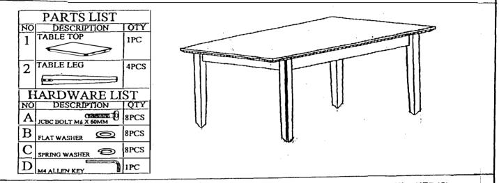
ATTACH THE TABLE LEGS (2) TO THE CORNER BLOCK WITH JCBC BOLT (A) SPRING WASHER (C) AND FLAT WASHER (B). TIGHTEN THE JCBC BOLT (A) BY USING ALLEN KEY (D)
