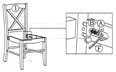
Use alien key (F), JCBC screw 50MM (A), spring washer (B) and flat washer (C) to assemble left and right side apron to chair back (#1). Tighten all screws.
