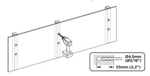
• Secure the mount to the wall using the Lag Screws (#L) and tighten the screws until secure.
