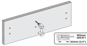
• Insert the Concrete Anchors (#M) into the holes then secure the mount to the wall using the Lag Screws (#L) and tighten the screws until secure.
