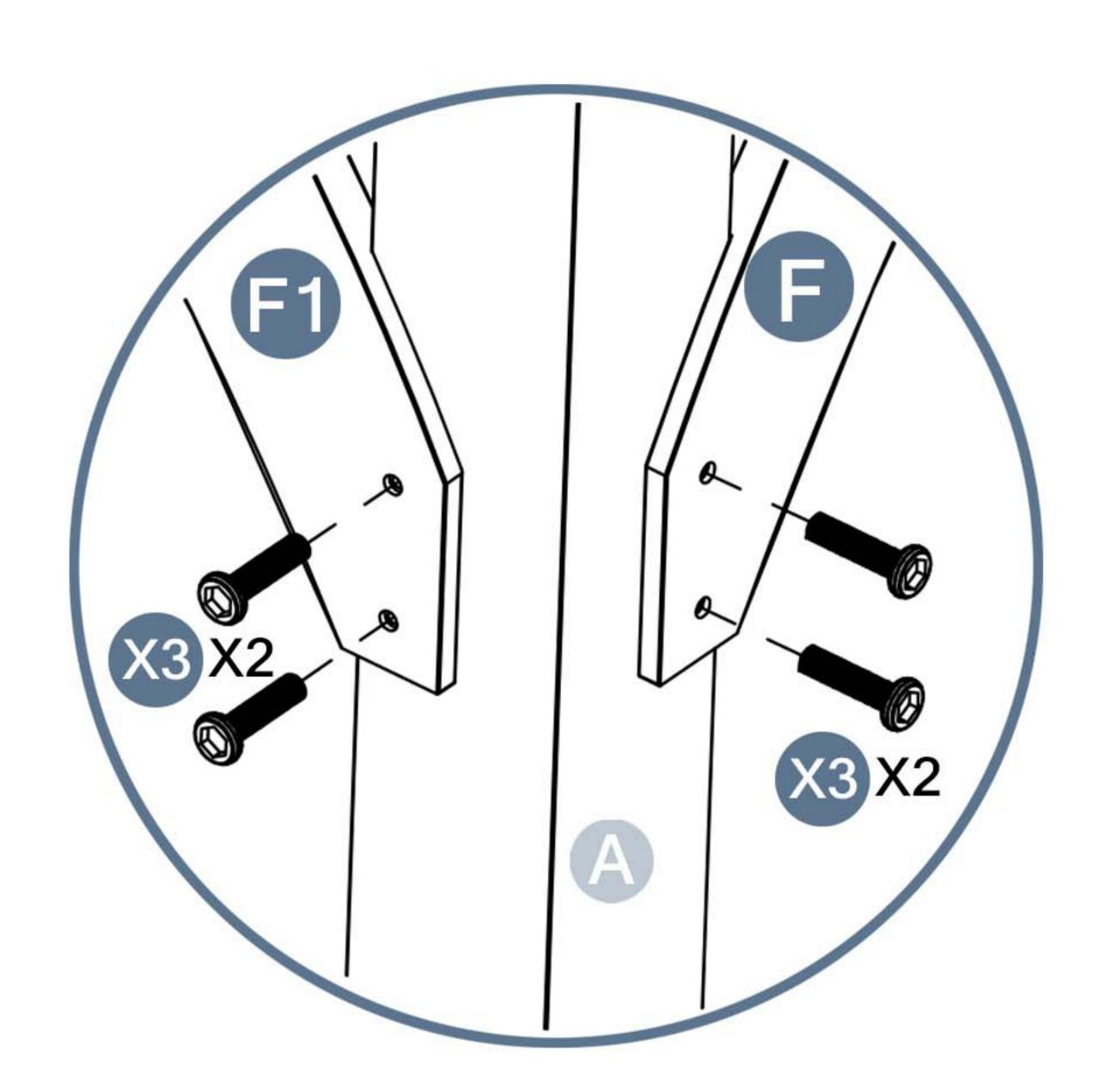
When installing F and F1, please note that the top is on the inside and the bottom is on the outside.
