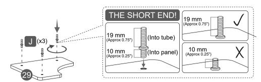
• Attach the tubes 28 to the LONG END of the screws J.
