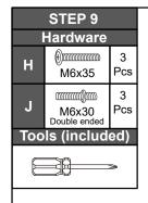
• Install the SHORT END of the screws J into panel 29.
