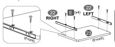
The sliders #22 have only 2 or 3 threaded holes; if the sliders you are trying to install have lots of holes with no threads, then you are using the wrong sliders #4 and you must go back to STEP 2 and swap these sliders.
