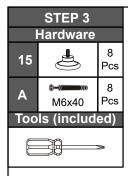
• Attach the glide stude 15 to the underside face of the bottom panels 13 & 20. The surface of the panels will have only 4 visible holes.
