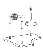
• Attach the tubes 28 from the shelf 29 to the tabletop 24 with screws H.
