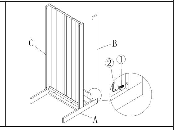
Attach the Back Support Bar(B) to the Side Panel(A) using Bolt(1) with Allen Key(2). **Do not fully tighten Bolt.**
