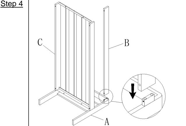
Insert the Back Support Bar(B) into the Side Panel(A).
