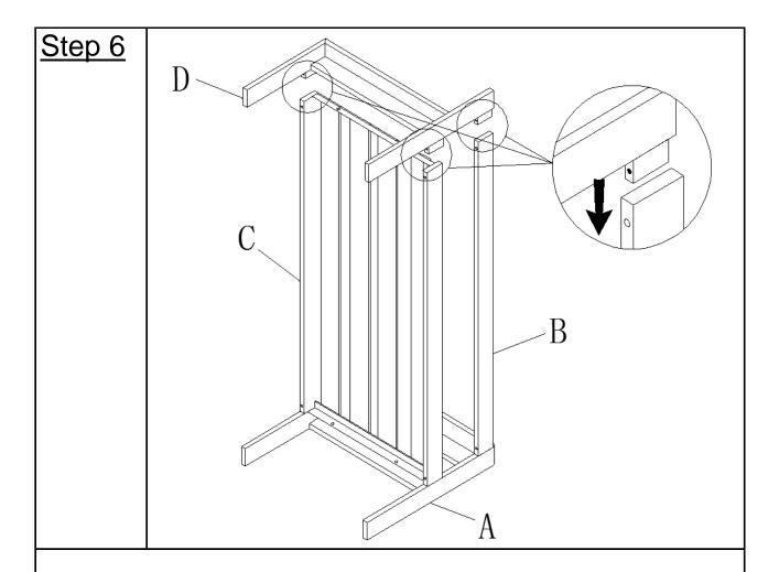
Insert the Leg Support Bar(D) into the Back Support Bar(B) and Seat Panel(C) as shown above.
