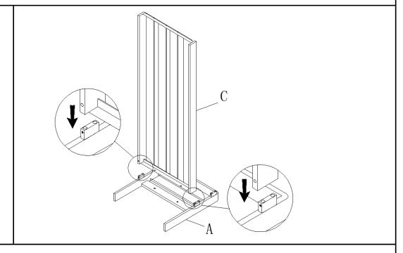
Place the Side Panel(A) with its inside facing up. Insert Seat Panel(C) into the Side Panel(A).
