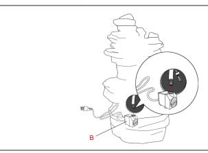
Connect and insert the pipe into the Pump (B) showed as above.
