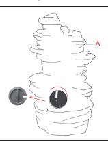
Place the fountain on a level surface away from areas where it is likely to get colgged with leaves and make sure that the cable will reach the socket and open the back door(anticlockwise).
