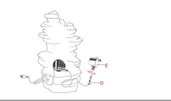
Connect and insert the Splitter(D) to Transformer(E).
