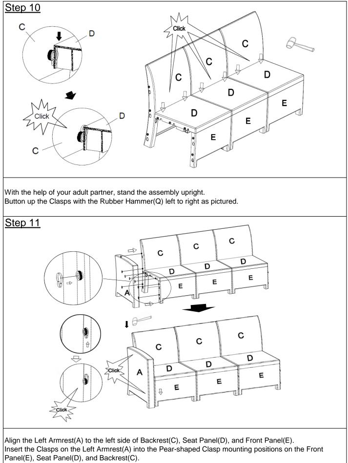
Insert the 8 Clasps of Front Panel(E), Seat Panel(D), and Backrest(C) into Pear-Shaped Clasp mounting positions of Left Armrest(A).
