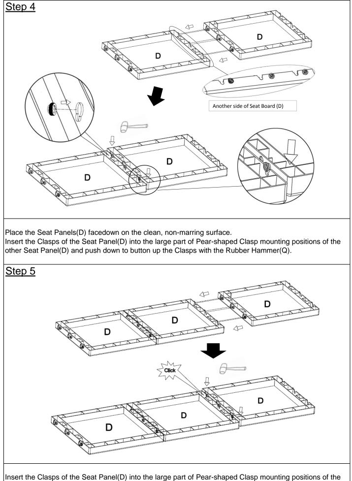
other Seat Panel(D) and push down to button up the Clasps with the Rubber Hammer(Q).
