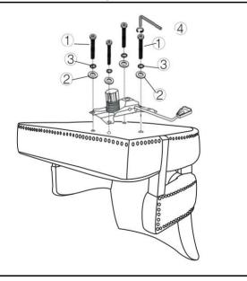
Attach Mechanism(B) to Chair Seat(A) using Bolts(1), Washers(2), and Spring Washers(3) with Allen Key(4).
