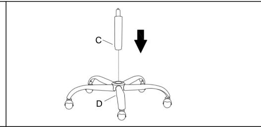
Insert the Gaslift(C) into the mounting position under of Chrome base(D) as pictured.
