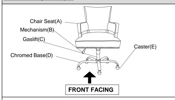
This Office Chair has multiple parts and may require up to 30 minutes to assemble. To give you an overview of the Office Chair parts, the above picture is to help you put the various parts into perspective. Please read through the instructions below to familiarise yourself with the parts and steps before assembly.
