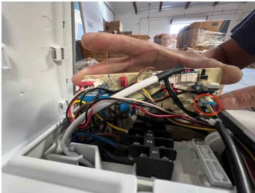
Step 4: Attach WiFi to the inside of front panel:
