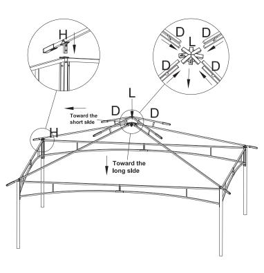
Step 4:Insert four Part H to the four corners of the frame (the top of Part A) .
