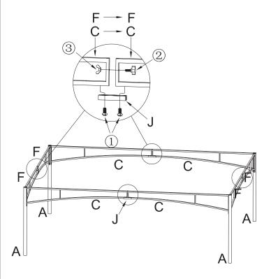
Step 2:Use Nut③ and Srew② to connect two Part C(or Part F),and tighten them. Then put one Part J on the bottom side of two attached Part C(or Part F).Use Screw① to tighten the Part J.
