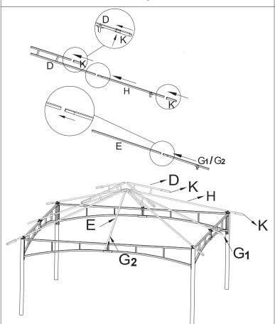
Step 3: Insert the small head of Part H to the long side of Part D directly and insert one Part K to the other head of Part H. Then insert one Part K to the short side of Part D.Insert the small head of Part G1 or G2 to Part E.
