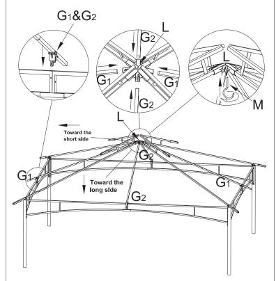
Step 5:Insert Part G1 to the connection part of the two attached Part F. Then Insert Part G2(the shorter piece) to the connection part of the two attached Part C.Next insert Part E to Part L.
