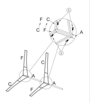
Step 1:Put Part C and Part F together and put the Part A in the middle of them,then use Screw① to tighten them.
