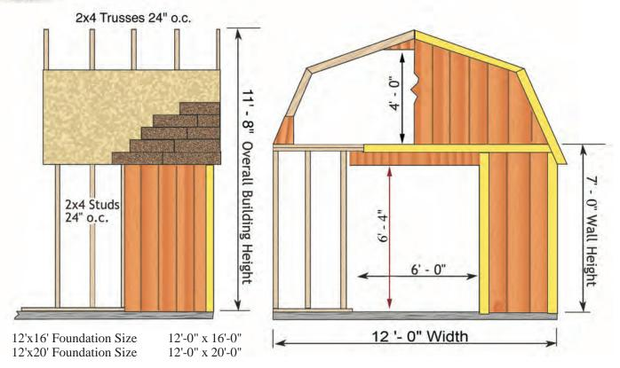
**Wall Framing:** 2x4 Construction with 24" on center stud spacing, single bottom plate and top plate with 2x4 tie plates.
