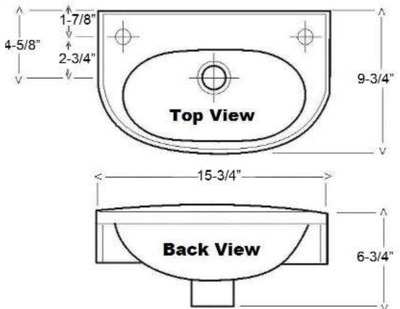
Dimensions of fixture are nominal and may vary within the range of tolerances established by ASME Standard A112.19.2. Dimensions and specifications subject to change without notice.
