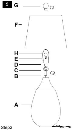
Insert the Harp (E) into the Saddle (C). Put the shade(F) on the Harp(E),then tighten the Finial (G)into the Harp (E) Insert the bulb(H) into the socket(D).
