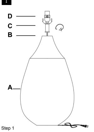
Pull power cord to connect the Neck (B) to the Base (A). Screw the Neck (B) onto the Lamp base (A) Be careful not to twist the power cord and tighten securely
