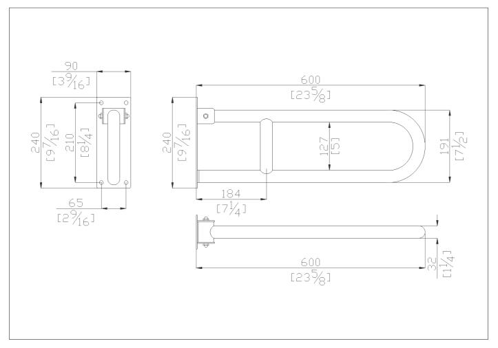
Folding grab bar made of seamless stainless steel AISI 304 pipe, with satin finish
