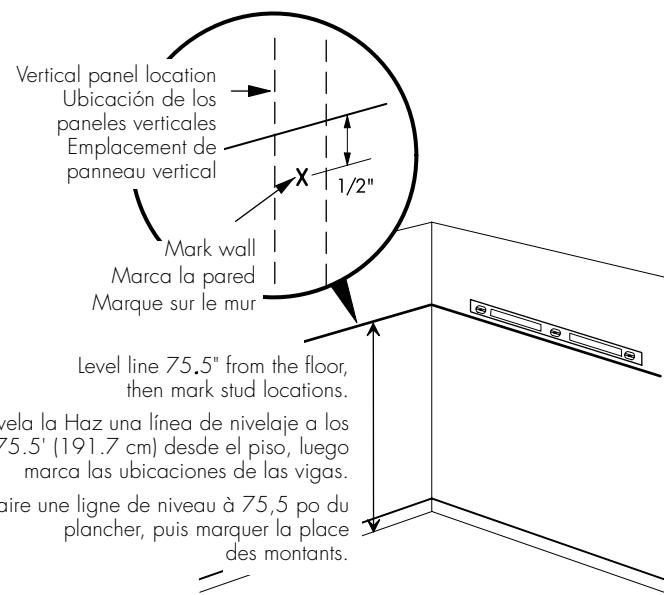
**2** Locate studs. Tap the wall or use an electronic stud finder to locate studs. Mark wall  $\frac{1}{2}$ " below horizontal line. Studs (2 x 4) are usually located on 16" centers measured from the left or right side.
