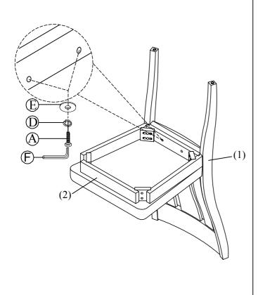
STEP.2 Attach the seat frame to the chair back using long bolt (C), spring washers (D), flat washers (E), and allen key (F).
