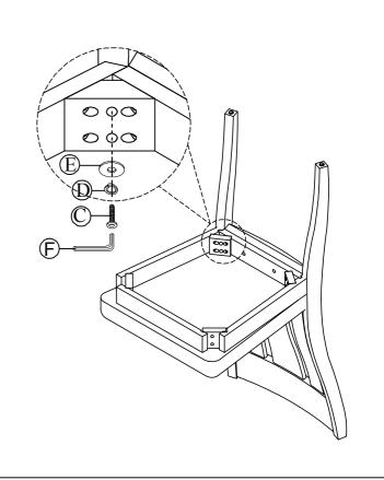
STEP.3 Attach the front legs to the seat frame and using medium bolts(B), spring washers (D), flat washers (E), and allen key (F).
