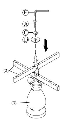
STEP.2 Attach Support rail to the table top and using long bolts (A), spring washers (C), flat washers (D), and allen key (E).
