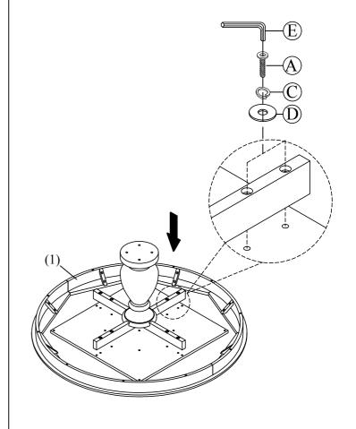
STEP.3 Attach base panel to Pedestal and using short bolts (B), spring washers (C), flat washers (D), and allen key (E). Attach foot to base panel by rotating it from left to right.
