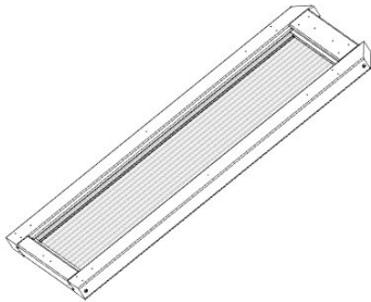
WA09 WINDOW ASSEMBLY - W2A04378 (x1) 1 7/16"x15 1/4"x35 1/4" (36x388x802)
