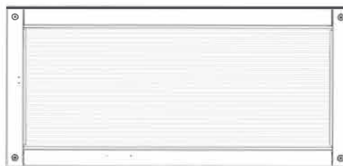
WA06 WINDOW ASSEMBLY - W2A04205 (x2) 1 7/8"x21 13/16"x47 3/16" (48x554x1198)
