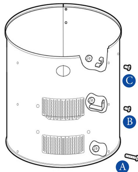
**D.** Align Handle Bracket (13) over one pair of holes near the top of the Body Assembly. Insert a 10-24 x 3/8" bolt (2) through each hole in the Bracket then through the Body. Fasten in place with a Lock Nut and tighten. Repeat for Handle Bracket on opposite side of Body Assembly.
