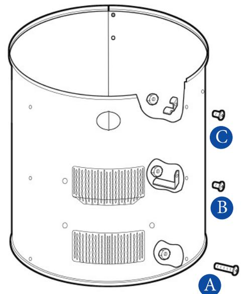
**D.** Align Handle Bracket (13) over one pair of holes near the top of the Body Assembly. Insert a 10-24 x 3/8" Bolt (2) through each hole in the Bracket then through the Body. Fasten in place with a Lock Nut (3) and tighten. Repeat for Handle Bracket on opposite side of Body Assembly.
