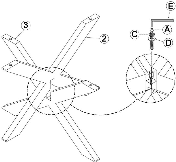
**STEP.2:** Attach the Connect Board (4) to the legs,then tighten with Short Bolt (B), Spring Washer (C), Flat Washer (D) and fully tighten with Allen key (E).
