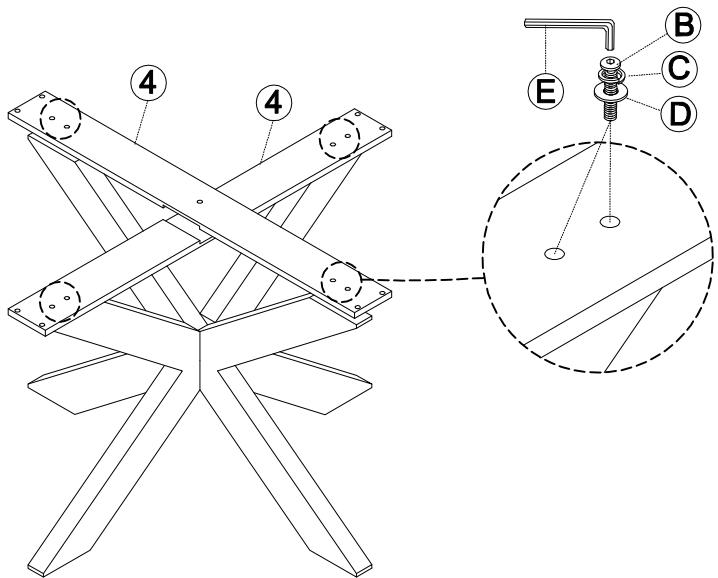
**STEP.3:** Attach the leg set to the table top (1),then tighten with Short Bolt (B), Spring Washer (C), Flat Washer (D) and fully tighten with Allen key (E).
