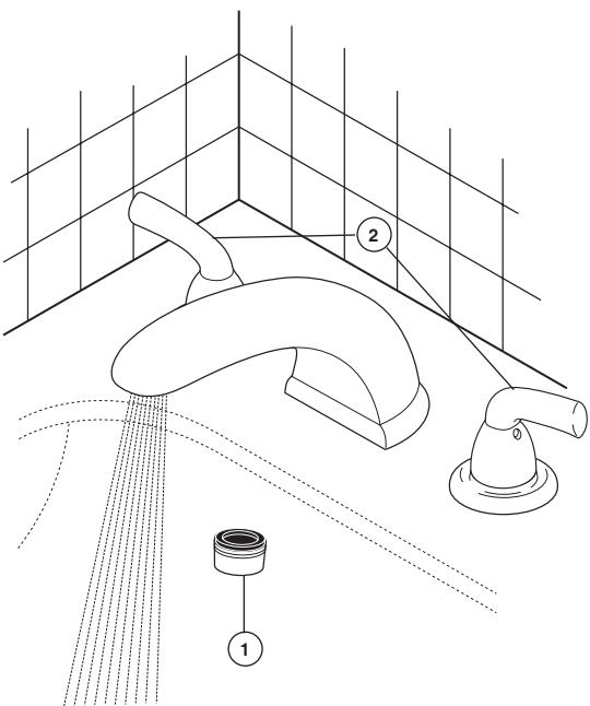
Remove Stream Straightener (1), turn faucet handles (2) all the way on. Turn on hot and cold water supplies and flush water lines for one minute.
