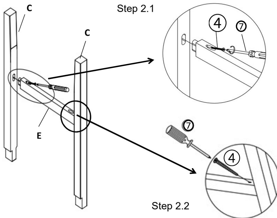
Attach Front Rail (E) into the housing of the Left Front Leg(C1) and Right Front Leg(C2).
