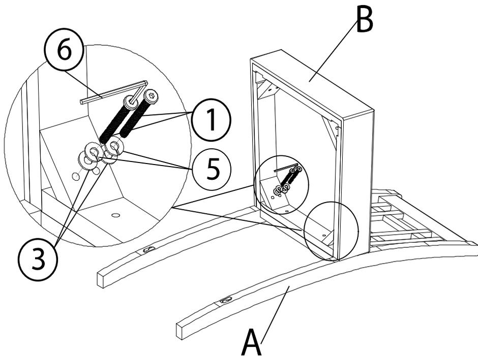
Secure Chair Seat(B) to the Chair Back(A), using Long Bolt(1) Spring Washer(5) and Flat washer(3) with Allen Key(6).
