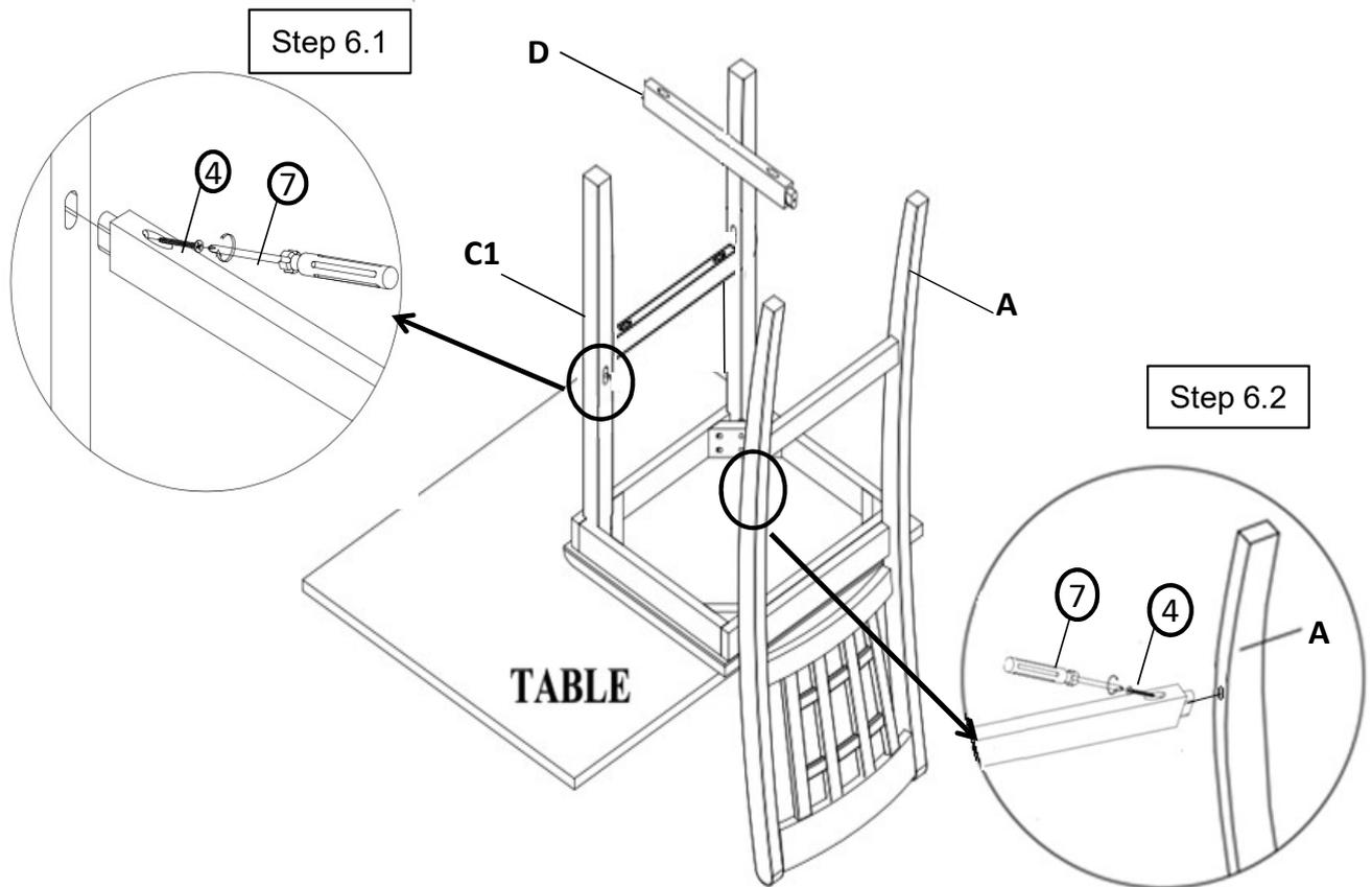
Next place Side Rail(D) into the housing of the Hind Leg of the Chair Back(A) and Left Front Leg(C1).
