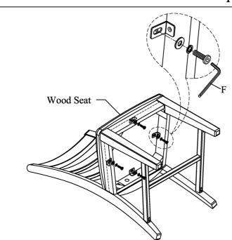
STEP 6. Unbolt bolt, lock washer and flat washer by allen key (F) and keep them well for re-use in step 7. Remove the wood seat.
