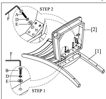
STEP 1. Place chair back (1) on a clean & padded surface then attach seat frame + wood seat (2) to the chair back using bolt (B), lock washer (D), flat washer (E), and tighten with allen key (F). Important: Do not over-tighten. STEP 2. Attach back assembly to the seat frame + wood seat (2) using bolt (A), lock washer (D), flat washer (E), and tighten with allen key (F).
