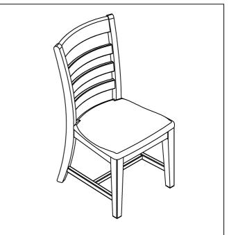
STEP 5. To ensure chair is stable, tighten bolts (A,B), using the allen key (F), tighten nuts (C) using spanner wrench (G), tighten screw (H) using the screwdriver while applying downward pressure to the seat.
