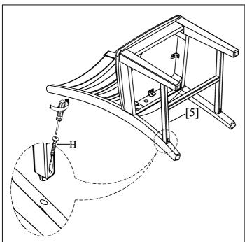
STEP 4. Attach the stretcher frame (5) to the back and front legs with screw (H) and tighten with screwdriver. Important: Do not over-tighten
