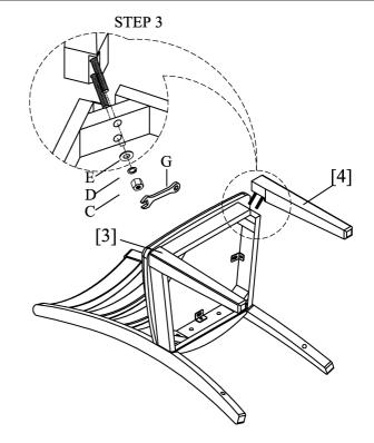
STEP 3 .Attach the left front leg (3) and right front leg (4) to the seat frame + wood seat (2) using nut (C), lock washer (D), flat washer (E), and tighten with spanner wrench (G). Important: Do not over-tighten.
