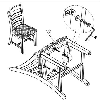
STEP 7. Assemble the seat cushion (6) to the seat frame by tighten bolts, lock washers, flat washers from step 6 with allen key (F).
