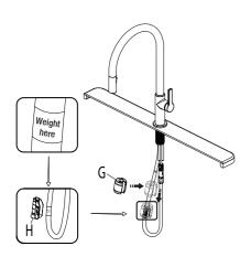
Install the weight clip (H) at the point of the hose marking "weight here". Insert the weight (G) onto the weight clip (H) by sliding it down onto the weight clip (H).
