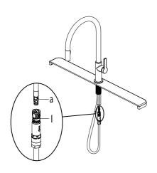
Push the quick connector (I) firmly upward and attach it to the receiving block (a). Pull down moderately to ensure the connection has been made.
