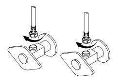
Attach waterlines to angle stops and tighten until snug. Turn on angles stops and check for leaks (DO NOT TURN FAUCET ON)
