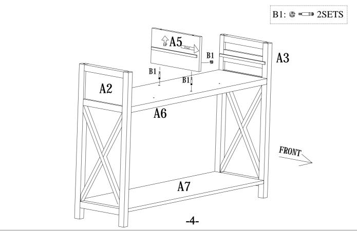
Step 4: Assemble top panel A1 to the side frames A2, A3 and divider A5 using camlocks B1.
