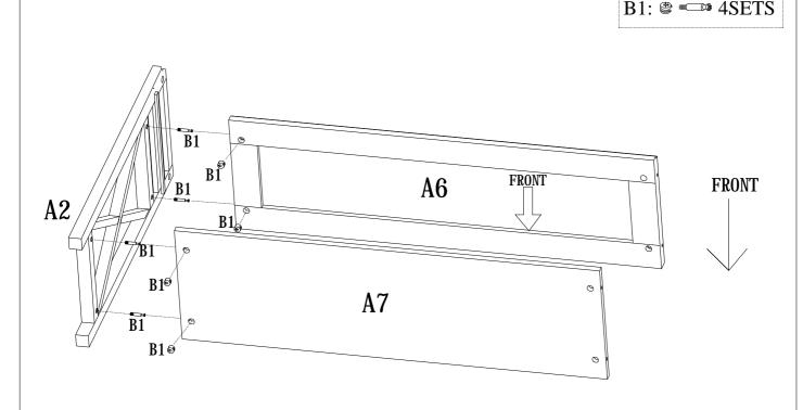
Step 2: Assemble the middle shelf A6& bottom shelf A7 to the other side frame A3 using camlocks B1.
