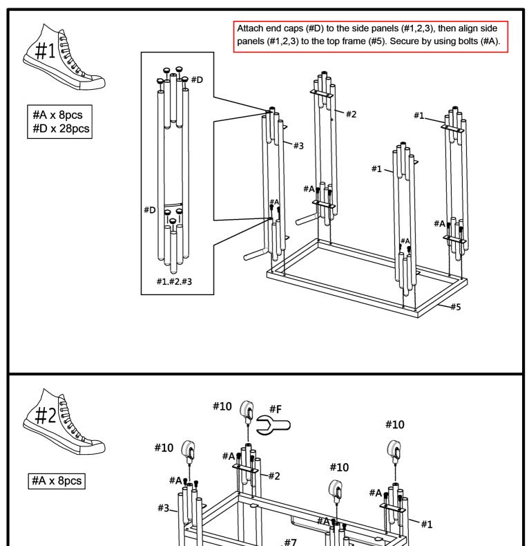
Align bottom frame (#7) to the side panels (#1,2,3), then secure by using bolts (#A). Align wheels (#10) to the holes of the side panels (#1,2,3), then secure by using wrench (#F) onto the hex nut of the wheel (#10).
