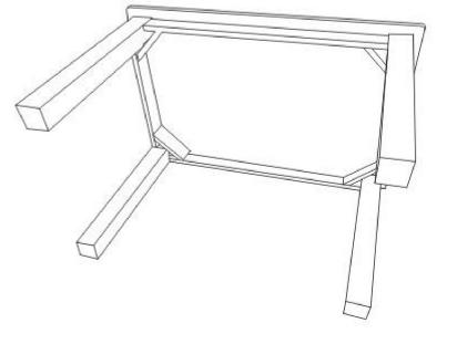
Step4. : Finish fixing and turn the table around.
