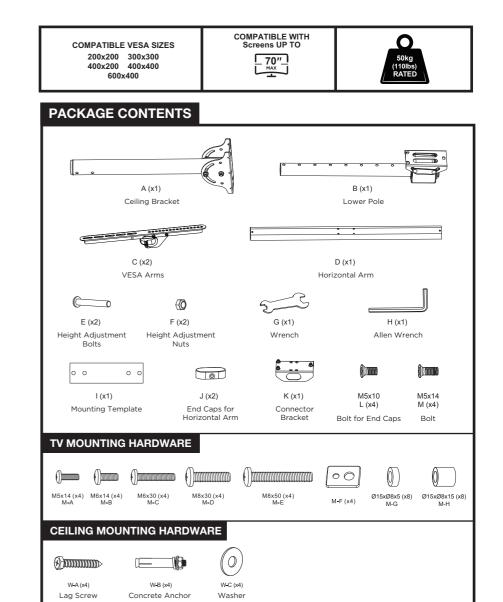
Check carefully to make sure there are no missing or defective parts. Some hardware provided may not be used. Use the correct wall mounting and monitor mounting hardware suitable for your installation.
