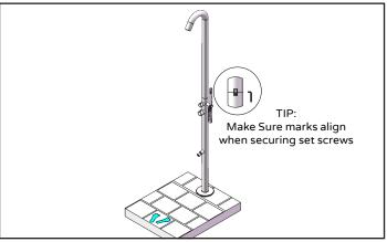
Insert top shower pipe (1) into bottom shower pipe (2). Connect hex head end of hose to swivel joint and tapered end to handshower (4). Place the tapered end of the hose into the handshower holder (9).
