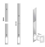
**Step 4:** Close your window to secure the kit in place. It needs to hold the windows kit firmly in place, and secure the window kit with duct tape if required. It is recommended that the gap between the adapter and the sides of the window should be sealed off for maximum efficiency.
