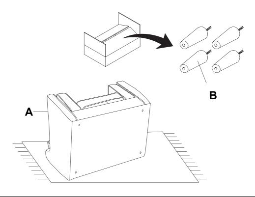
Tighten each Leg (B) in a clockwise direction.
