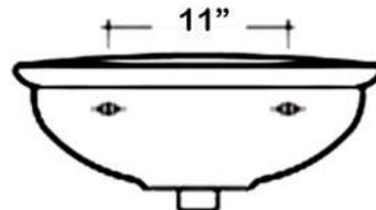
Dimensions of fixture are nominal and may vary within the range of tolerances established by ASME Standard A112.19.2.2013. Dimensions and specifications subject to change without notice.
