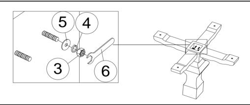
Place the Pedestal (B) and the Table Leg (C) on a carpeted surface. Attach the Table Leg (C) to the Pedestal (B) by inserting the Hex Nuts 5/16"x 18MM(3), Spring Washers 5/16"(4) and Flat Washers 5/16"(5). Tighten with the Spanner (R/B)12.8 (6) as shown in the picture.
