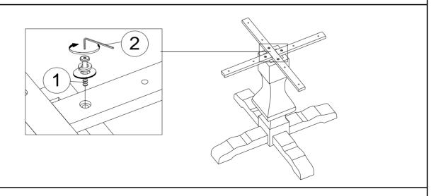
Cross the Table Leg Support (R&L)(D) as shown in Step 2.1. Then attach the Table Leg Support (R&L)(D) to the Pedestal (B) by inserting the JCBC BOLTS M6 x 30MM①,Spring Washers 1/14"① and Flat Washers 13MM①. Tighten with the Allen Wrench M4(Ball shape)Long②.
