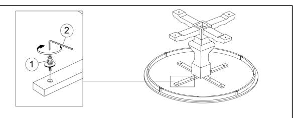
After that, stand the Pedestal (B) up and set it as shown in the picture. Then make sure the hole of the Table Leg Support (R&L)(D) align with hole of the Table Top(A) by inserting the JCBC BOLTs M6 x 30MM①, Spring Washers 1/14"① and Flat Washers 13MM①. Tighten with the Allen Wrench M4(Ball Shape)Long②. Finally, the assembly is completed.
