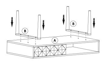
**STEP2** Place the table upside down on a clean surface. Align legs on both sides of table as per side holes present on either side of table.
