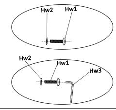
**STEP3** Put the washer on the Bolt in the order shown in picture.
