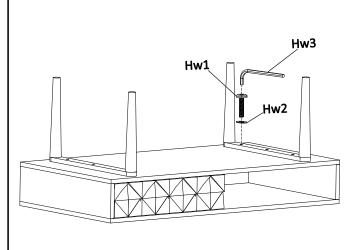
STEP4 Insert Allen Bolt (Hw1) with Washer (Hw2) tighten with Allen Key (Hw3).Don't over tighten.
