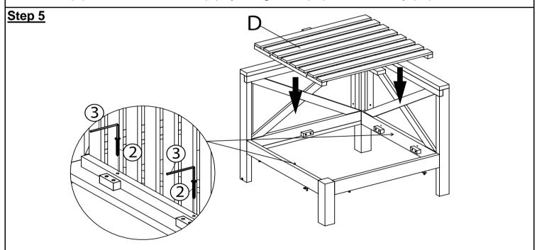
Attach the Seat Panel (D) into the Corner Chair as shown in picture above.
