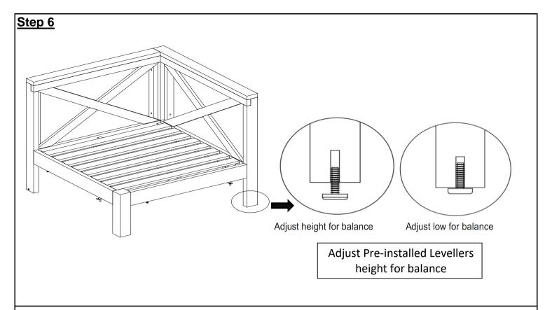
Inspect the Corner Chair and make sure all parts are adequately connected.
