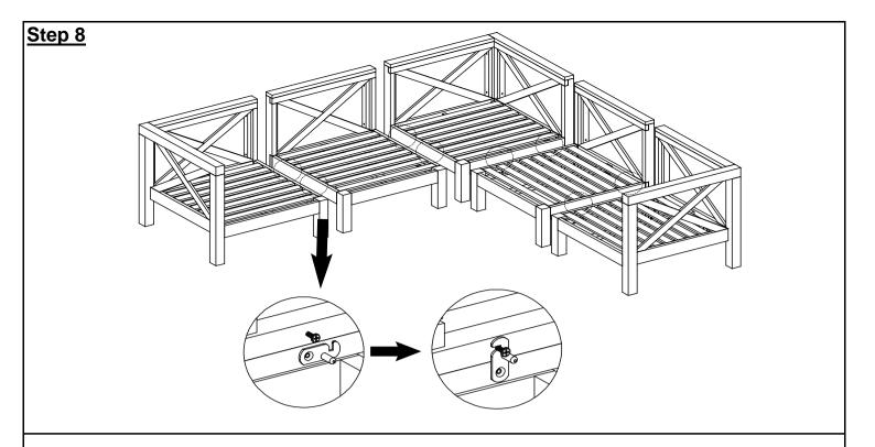
Note: This is optional step in case we want to connect all chairs in a set together and should be done before placing cushion
