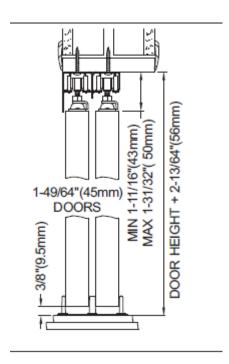
Refer to the diagram above to determine the height of the aluminum track. **Door height (i.e. 84") + 2-13/64"**
